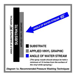
Under no circumstances should a turbo pressure nozzle be used when pressure washing applied vehicle graphics.
